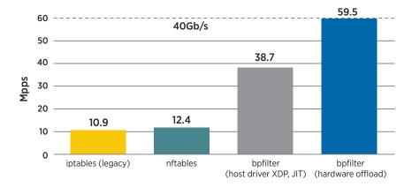
What becomes obvious is the remarkable performance improvement between bpfilter, iptables and nftables; a 3.5X improvement over iptables and a 3.1X improvement over nftables (~6X and ~5X respectively with hardware offload). More importantly, the test with transparent hardware offload provided line rate performance with zero impact to the host CPU, as the SmartNIC performed the processing needed to drop packets.
