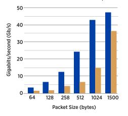
Agilio OVS Firewall Conntrack Performance vs. Software-based OVS Conntrack with Competitor NIC
