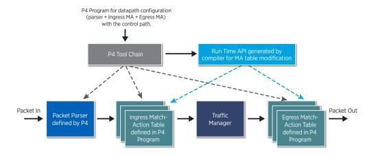
The SDK supports P4 syntax as defined on the P4 specifications published on P4 consortium website (www.p4.org). Netronome has integrated the open source P4 compiler in the SDK to generate an intermediate representation (App.IR) of the P4 program in the yaml format, which is further compiled by the P4 back-end compiler to generate a C program for the data path on the NFP. P4 programming support on the SDK is shown in the figure below.
