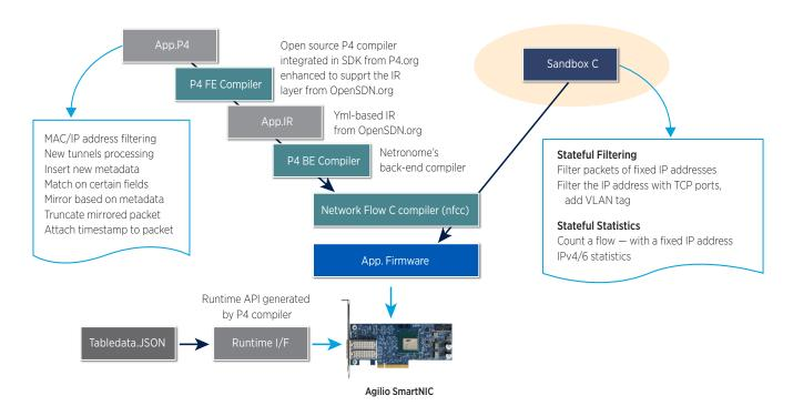
Since P4 is meant for hardware independent programming (flow processing), the user does
